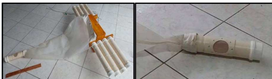
Figure 3: Low-cost Net for Microplastics and the collecting cup attached to the net.
