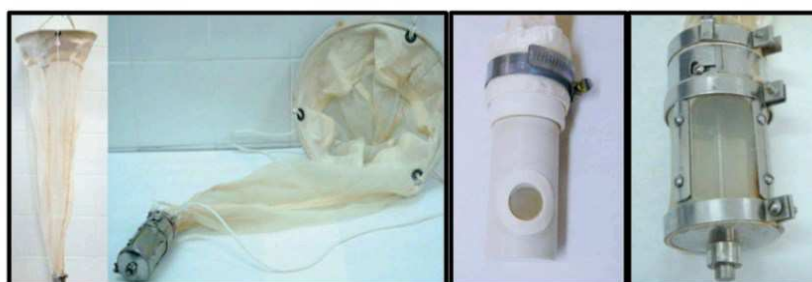
Figure 1: Nêuston net (sampling aquatic microorganisms) and collecting cups.
