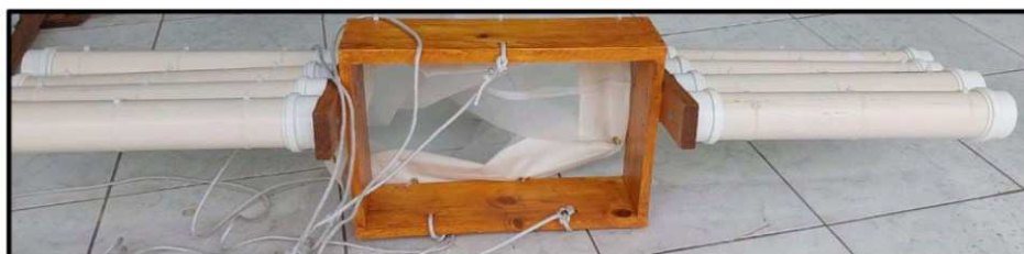
Figure 4: Front view of the Low-Cost Microplastic Net made of wood treated with marine varnish coupled with Neuston net and PVC pipes responsible for buoyancy.
