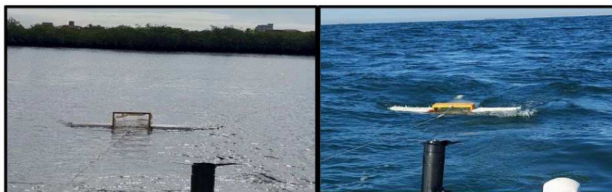
Figure 6. Sampling study using the Low-cost Net for Microplastics in fresh and marine waters.
