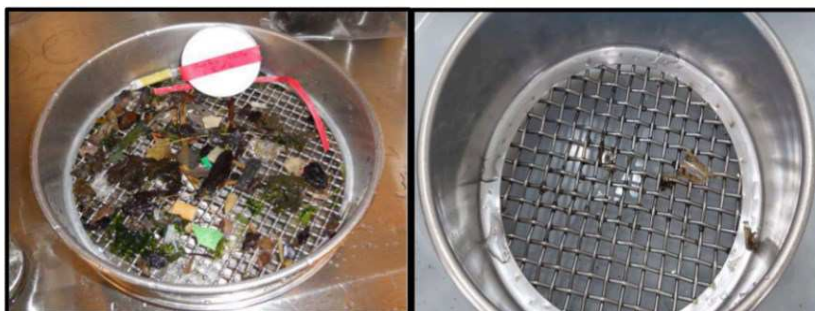
Figure 8. NOAA protocol sieve separation process and sample separation obtained after sampling by the Low-cost Net for Microplastics with fragments smaller than 5 mm.
